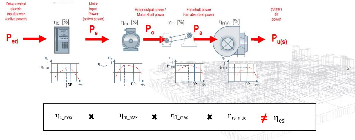
V-belt **AMCA 207 ISO 12759** Wire-to-air test Fan total efficiency in % Impeller shaft power in kW Belt efficiency in % Motor shaft power in kW Motor efficiency in % Wire-to-air efficiency in % Motor input power in kW
